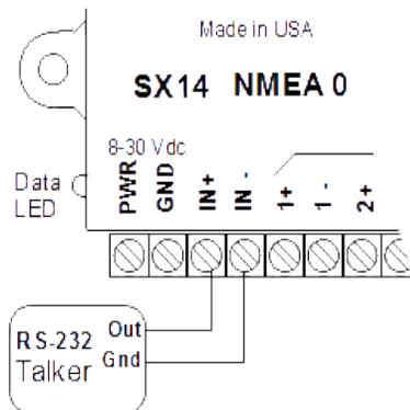
**LED Operation:** Two LED's are provided to verify proper operation and connection of the SX14. The green data LED flashes whenever input data is detected. When there is no data, the SX14 automatically switches into a low power “Standby” state, where it remains until data is again detected.
