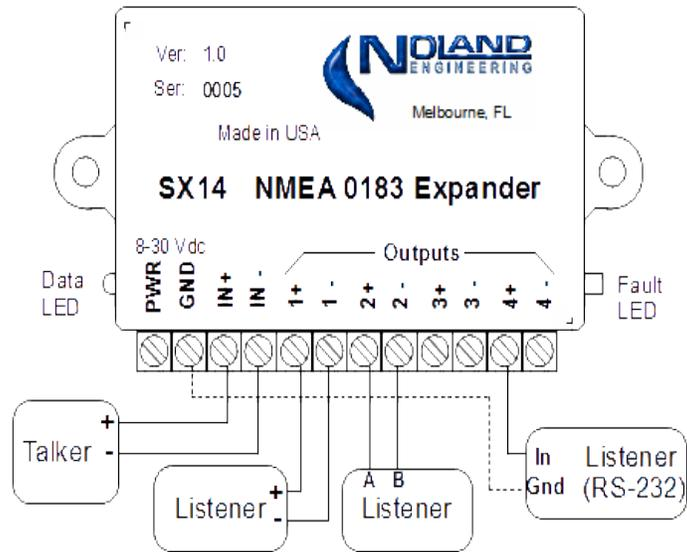
In the example, outputs 1 and 2 are connected to differential listeners that have “+/-” (or “A/B”) inputs which may also be labeled “A/B” or “RXA/RXB”. A third Listener (RS-232) uses only a “+” output from the SX14 to connect to the single input terminal “In”. The dashed “Gnd” wire may be needed in some installations for stable data, but is often not required.
