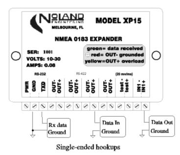
XP15 outputs one at a time, while observing that the LED never turns red. If one or more of the listeners causes the red LED to turn on, it is probably because that minus (-) listener input is actually grounded. In this case, you can either use the RS-232 output to drive that listener or leave the minus (-) input to that listener disconnected from the XP15. (See figure above.)
